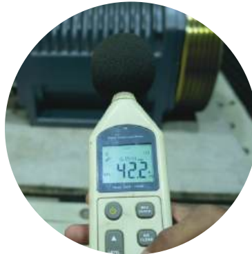
Noise proof room for noise test of PMSM
