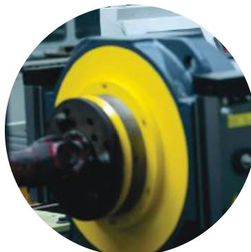
On-load PMSM testing
